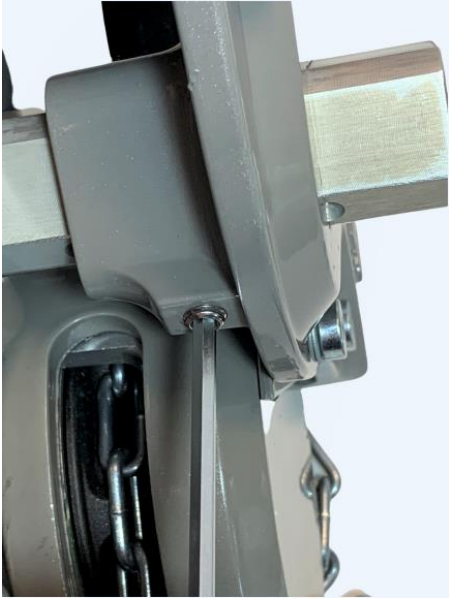
Pic. 10 Fasten the stop screw lightly with a 4 mm Allen key
