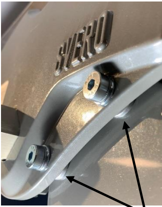
Pic. 4, 2x2,5 mm spacers for 120 mm beam
